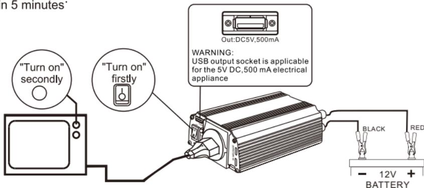
B) When connect the electrical appliance that with CRT,such as TV set, computer and so on to the Power Inverter which below 500W, the electrical appliance may be started for several times before it can work smoothly. Don't start the power inverter when it is with loaded, otherwise the power inverter will be damaged.
